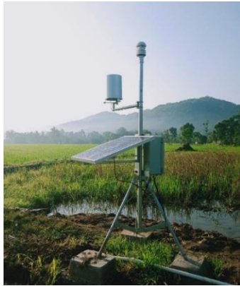
Gambar 2. Alat Pengukuran Automatic Weather Station (AWS)
